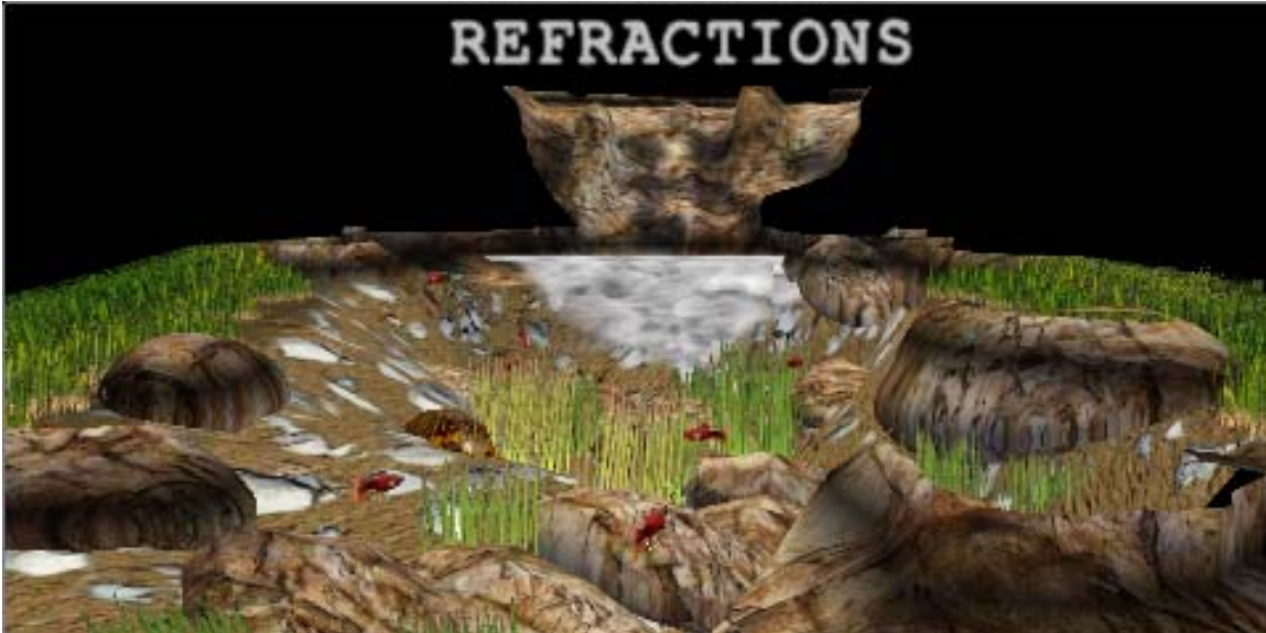
Figure 3 – Example of a refraction map created by drawing only the geometry below the water's surface.
