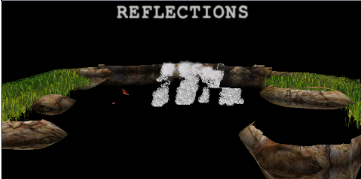
Figure 2 – Example of a reflection map created by reflecting scene geometry about the plane of the water's surface.
